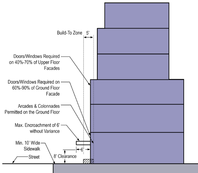
Figure 4.11.10. GMS Facade Elements
