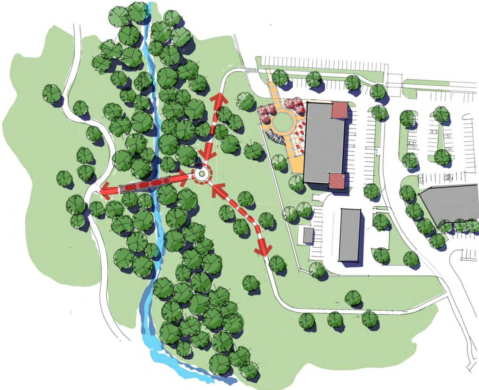
Example of making pedestrian connections between the fringes of development and natural features, emphasizing focal points for interest
